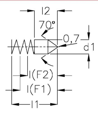
$\begin{array}{lll} \text{d1} & = 3.0 \\ \text{I(F1)} & = 13.0 \\ \text{I(F2)} & = 10.7 \\ \text{I1} & = 16 \\ \text{I2} & = 8.5 \\ \text{Spring pressure (F1) N = 4.8} \\ \text{Spring pressure (F2) N = 8.4} \end{array}$
